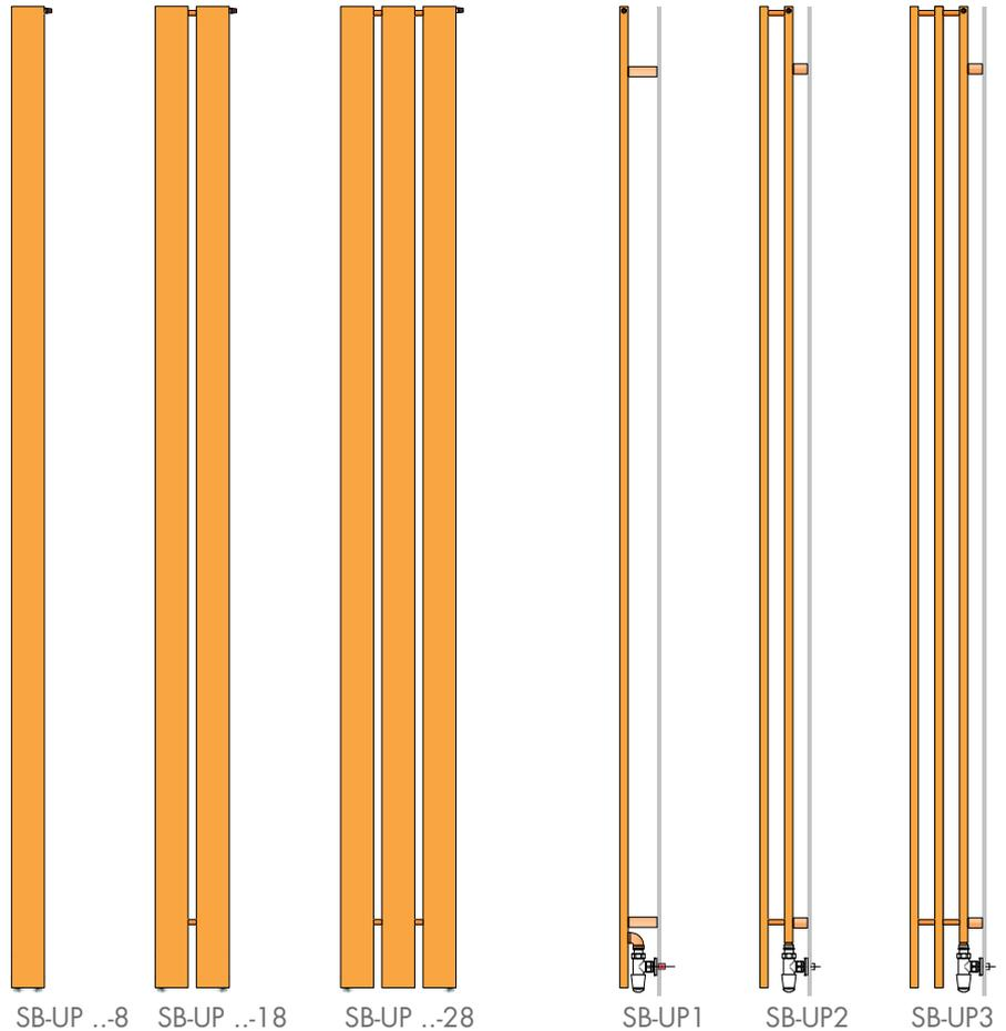
EN 442 Watt  $\Delta t$  50K ( $\Delta t$  40K =  $W \times 0,755$ ) ( $\Delta t$  30K =  $W \times 0,526$ )
